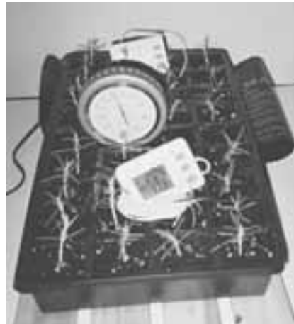
Temperature and humidity measurements on heated and unheated portion of trays during propagation experiments in Kamloops.
