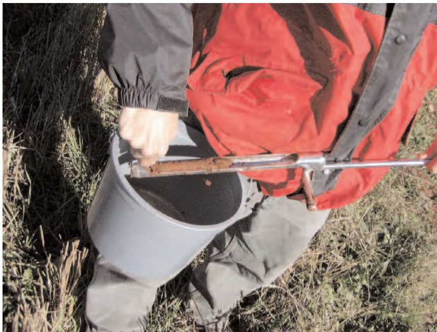
OACC research assistant, Alain Joseph, samples the soil in the fall after harvest. The depth of the soil probe is approximately 15cm. Twenty or more soil cores of a given area are combined to form a composite sample, then mixed and a representative subsample is submitted for testing.
