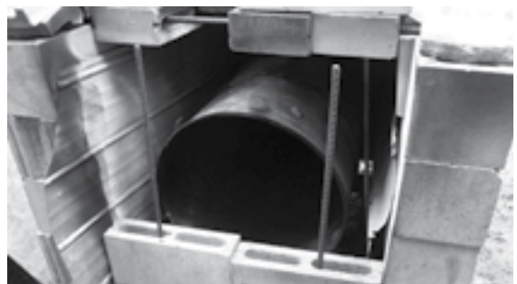
Above: The diagram of Fraser Common Farm’s biochar kiln. Below: The kiln uses pyrolysis to create biochar from a variety of fodder.
