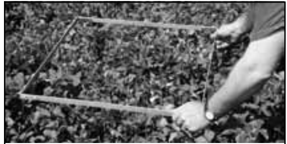
Figure 2. Placing the sampling frame (step 2).
